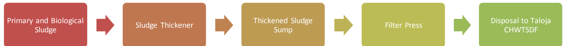
Figure 7-1: Process Treatment Line – Roha CETP Recommended Option
